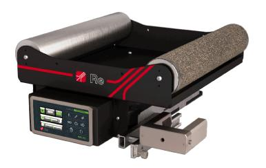
Moreover, in the plastic production process it is required to align and read the width of the plastic film. Thanks to the motorized sensor holders with encoder and driver integrated on the stepping motors, we ensure precision and quickness for the positioning of the sensors. It can be used both for edge control, center control or web width reading using infrared, ultrasonic or optical sensors.
